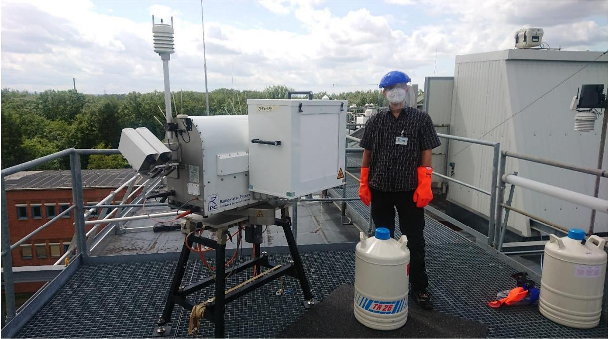
Figure 3: Equipment for LN2 calibration
