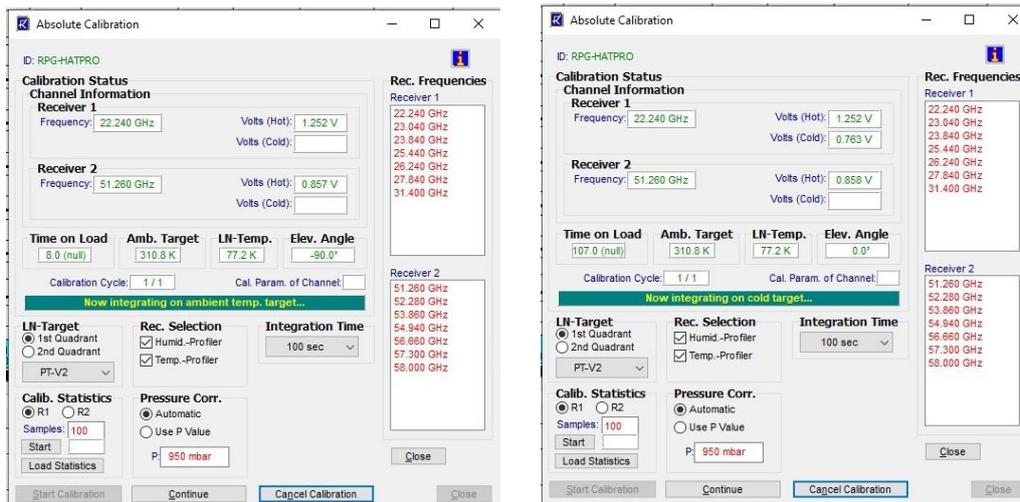
Figure 8: Absolute calibration window during LN2 calibration
