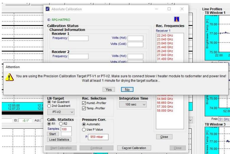
Figure 7: Pop-up window at absolute calibration to make sure that target surface is dry
