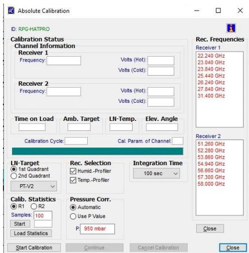
Figure 6: Software preparation for Liquid nitrogen calibration
