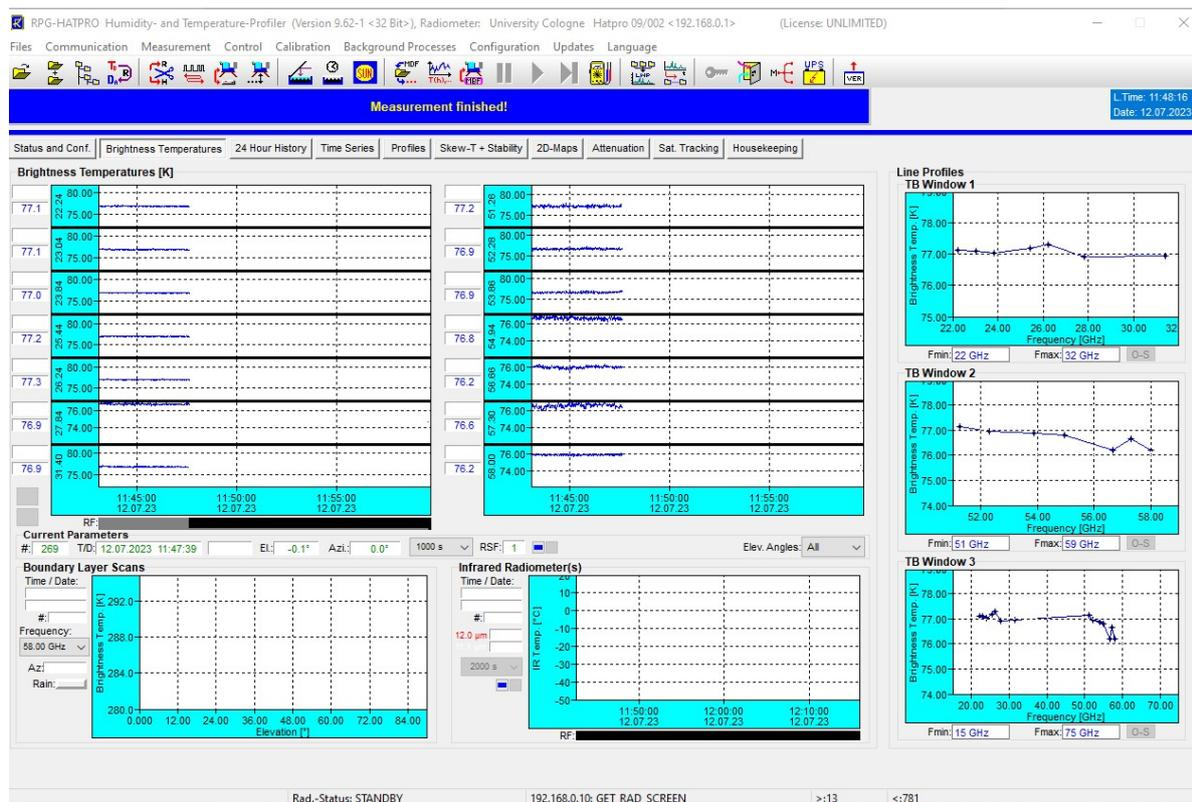
Figure 5: Measurement of LN2 observations finished. Note that all TBs should lie around the boiling point of liquid nitrogen (~77 K).
