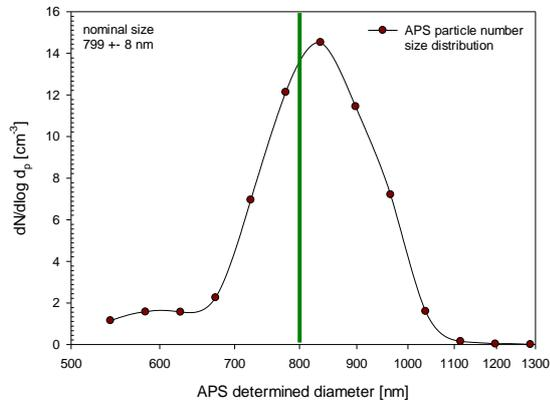
Figure 2e: APSS – 799 nm Latex particles
