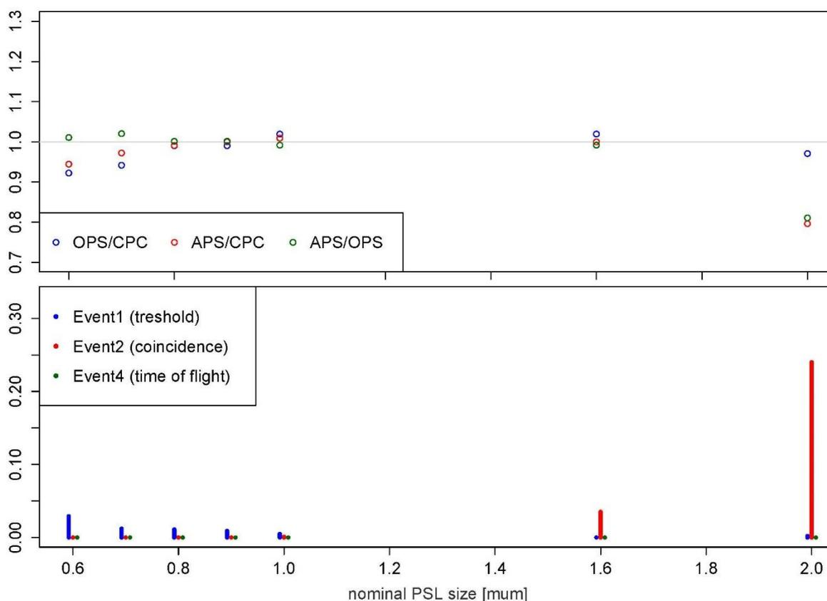
Figure 1: The upper part of the plot shows the counting efficiency of the APSS and OPSS against the CPC. Generally, for the size range from 0.6 to 1.0  $\mu\text{m}$  an acceptable efficiency of 100 +/- 10% was determined for all instruments. Only for 2.0  $\mu\text{m}$ , the counting efficiency was lower. The lower part of the plot explain the reason for the APSS, coincidence was the problem.
