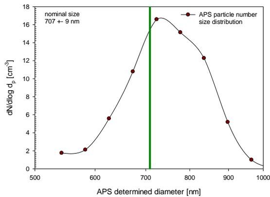
Figure 2c: APSS – 707 nm Latex particles
