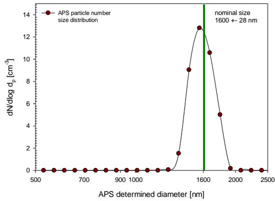
Figure 2k: APSS – 1600 nm Latex particles
