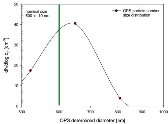
Figure 2b: OPSS – 600 nm Latex particles
