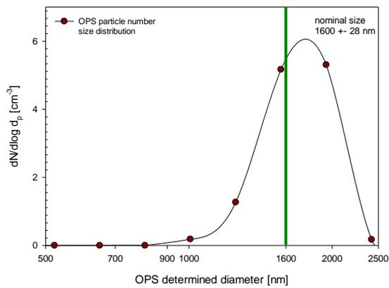
Figure 2l: OPSS – 1600 nm Latex particles
