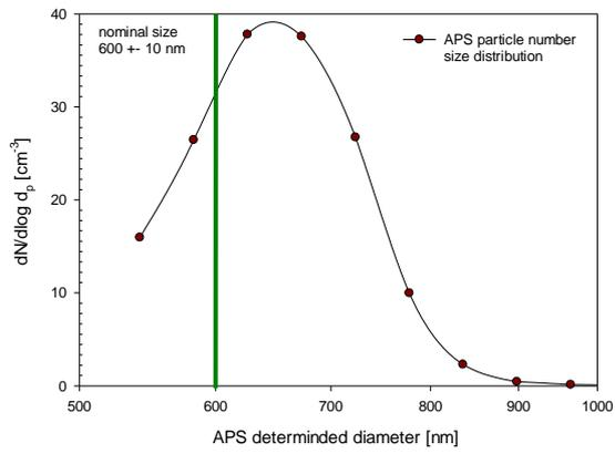
Figure 2a: APSS – 600 nm Latex particles
