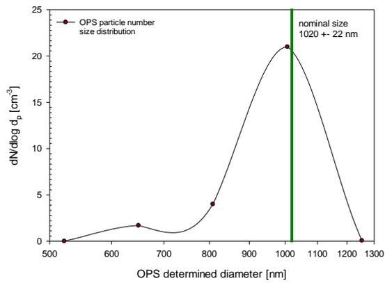
Figure 2j: OPSS – 1020 nm Latex particles
