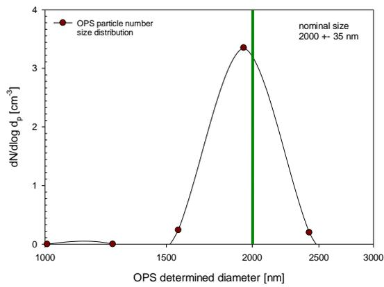
Figure 2n: OPSS – 2000 nm Latex particles
