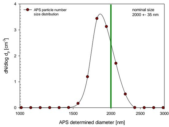
Figure 2m: APSS – 2000 nm Latex particles
