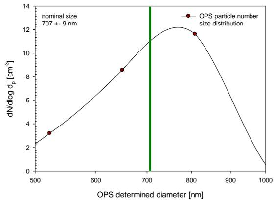
Figure 2d: OPSS – 707 nm Latex particles
