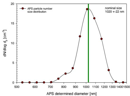
Figure 2i: APSS – 1020 nm Latex particles
