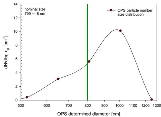
Figure 2f: OPSS – 799 nm Latex particles
