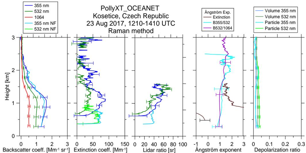
Figure 3: Multiwavelength optical products derived from PollyXT on 23 Aug 2017.
