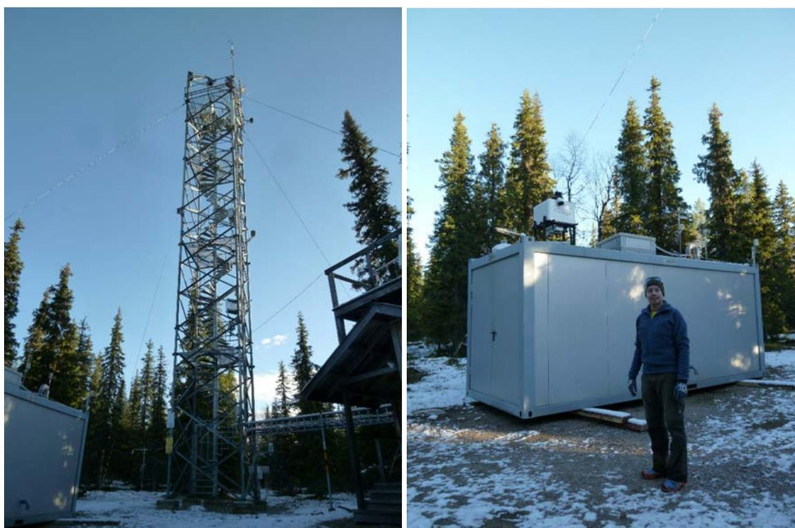
Figure 88. Instruments deployed at Kenttäröva, in northern Finland for the PACE2015 campaign. The tower (left) extends above the tree canopy, PollyXT and Halo Streamline Doppler lidar were operated within 2 m of each other.
