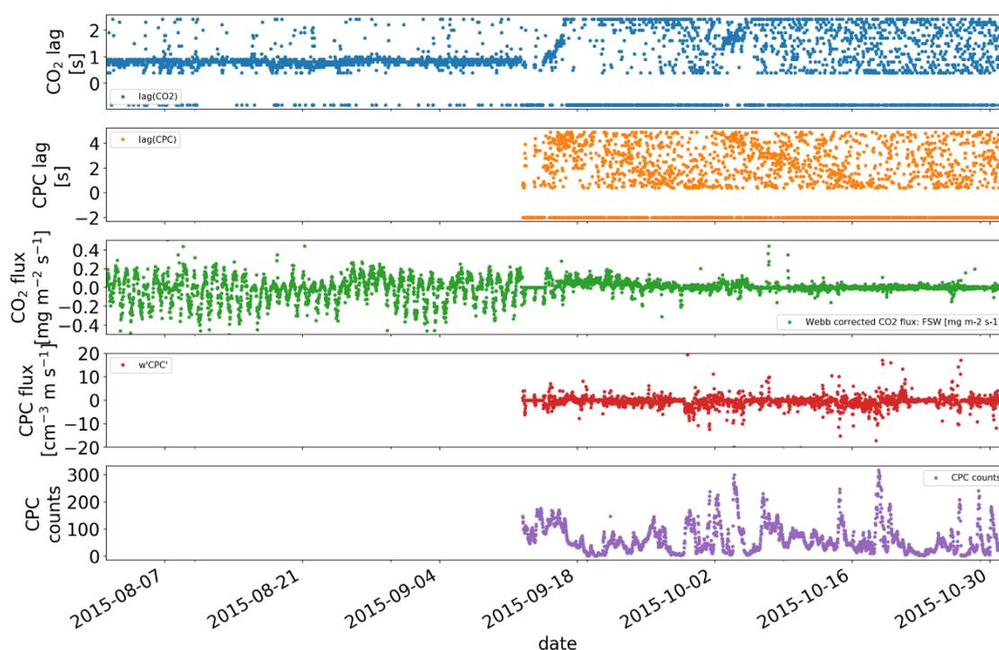
Figure 10: Flux measurements at Kenttäröva station (Pallas) before and after introduction of the CPC on 18<sup>th</sup> September 2015. Upper two panels display calculated lag time for carbon dioxide (CO<sub>2</sub>) and CPC measurements, centre panel displays CO<sub>2</sub> flux, lower two panels display CPC flux and CPC counts.
