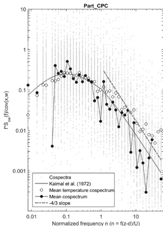
Figure 5. Mean cospectra of vertical wind speed and aerosol particle concentration calculated over April – August 2016. The measurements were made with the new measurement setup at the height of 35 meters.
