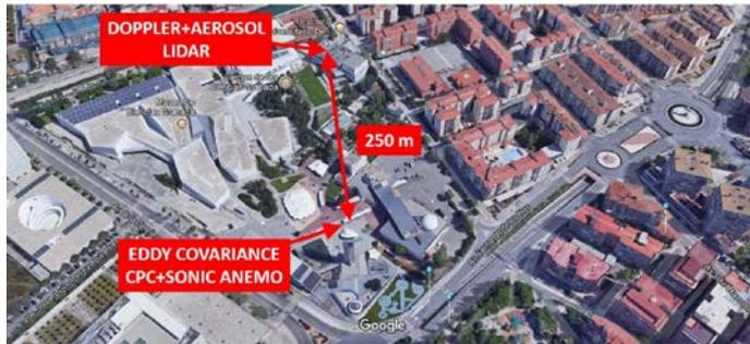
Figure 1. Experimental set up for the eddy covariance and remotes sensing setups at the urban area of Granada.
