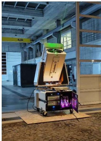
Figure 10: The eVe lidar system developed by Raymetrics for the validation of Aeolus.
