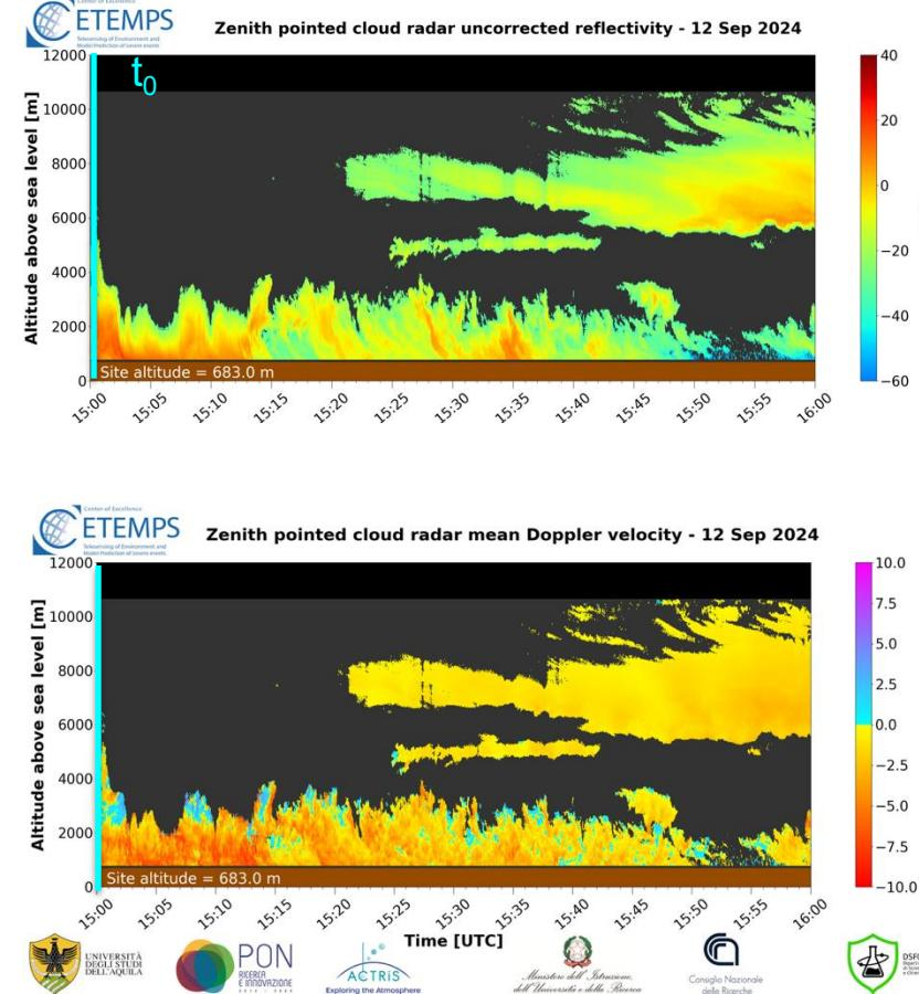
Mie notch is not always detectable, so vertical air profile may result incomplete especially in convection
