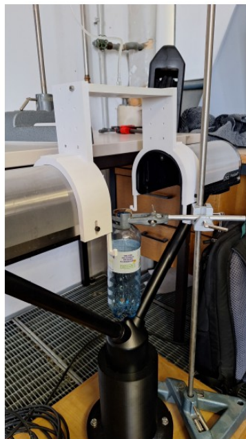
(c) Hole plate with end of tubing and collector bottle
