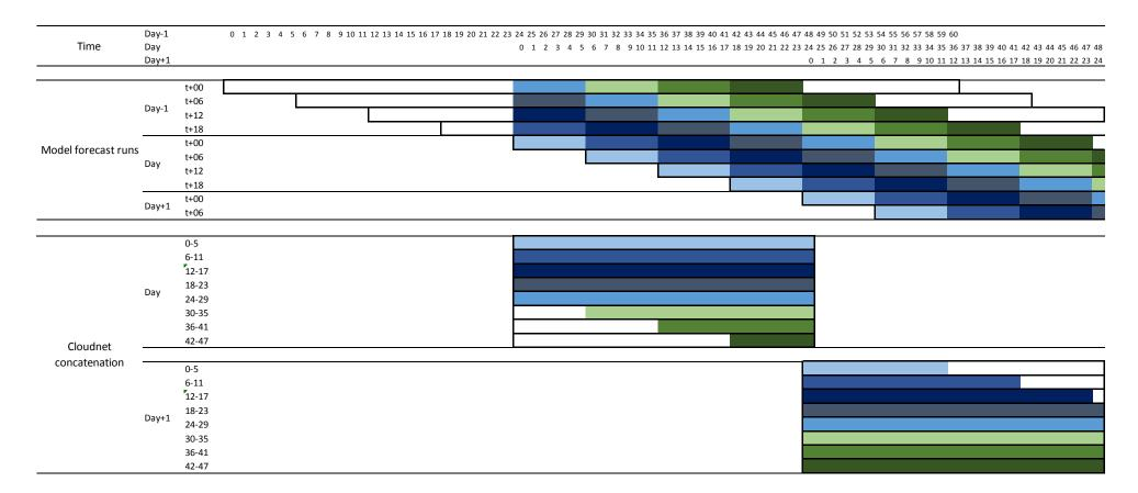
**Figure 2**: Model forecast concatenation within Cloudnet (for NWP model initialised 4 times a day: 00Z, 06Z, 12Z, 18Z). Each colour refers to a particular forecast window of 6 hours duration given in the 3<sup>rd</sup> column for the "Cloudnet concatenation" rows. These forecast windows are selected from sequential model forecast runs initialised every 6 hours as shown in the third column for rows in "Model forecast runs".
