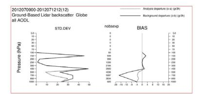
Figure 3. Ground-based LIDAR observations minus analysis (dash), forecast (solid) standard deviation (left) and bias (right) over all stations. The data are assimilated for 4 days (9<sup>th</sup> to 12<sup>th</sup> July 2012). Units for the horizontal axis are 10<sup>-7</sup> (sr.m)<sup>-1</sup>.
