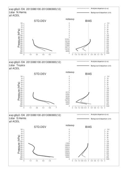
Figure 1. CALIOP observations minus analysis (dash), forecast (solid) standard deviation (left) and bias (right) for the north hemisphere (top), tropics (middle) and South hemisphere (bottom). The data are assimilated for 8 days (01<sup>st</sup> to 8<sup>th</sup> August 2013). Units of lidar backscatter are 10<sup>-7</sup> (sr.m)<sup>-1</sup>.
